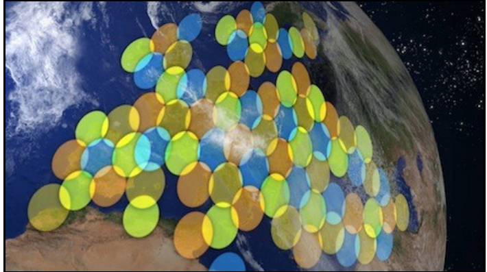
Spot Beam Pattern for Eutelsat's KA-SAT
